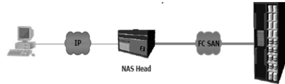
**Figure 2.2 Gateway NAS Architecture**
