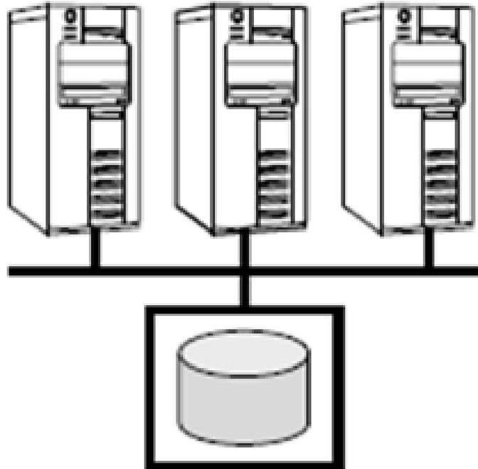
**Figure 2: Network Attached Storage**
