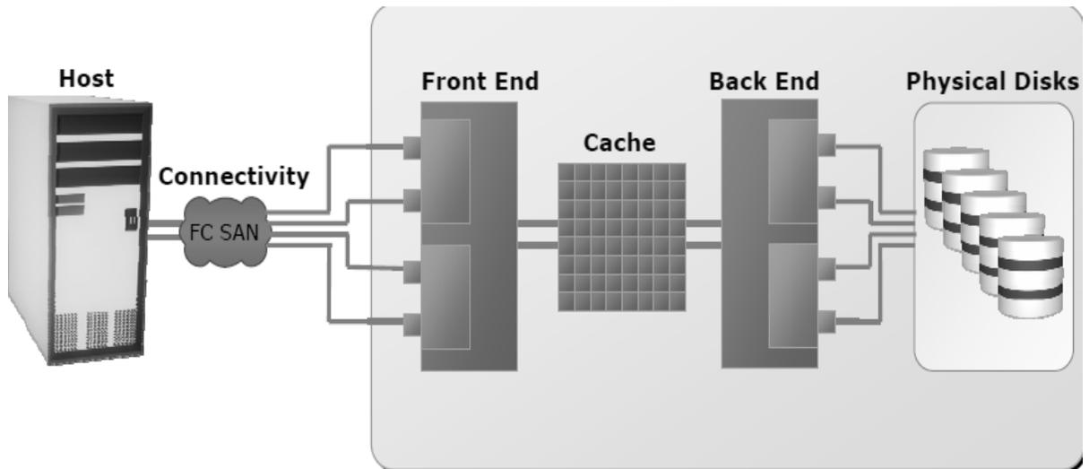
Figure 3.1 EMC Symmetrix Architecture
