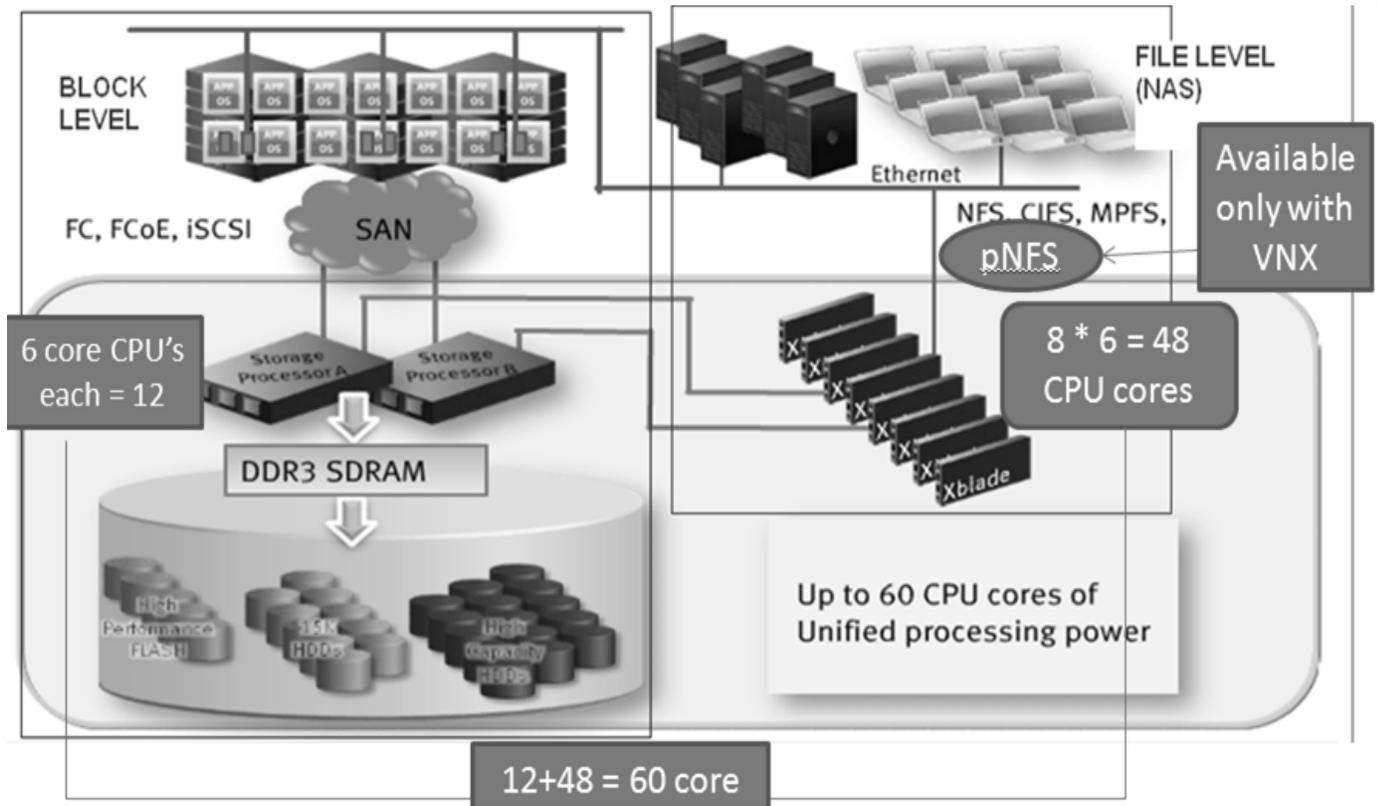
Figure 4: Unified Storage Architecture
