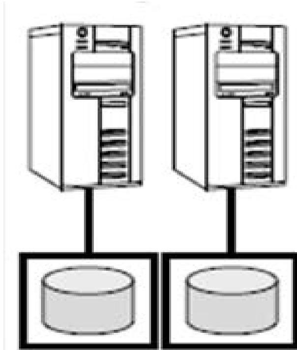
**Figure 1: Direct Attached Storage**
