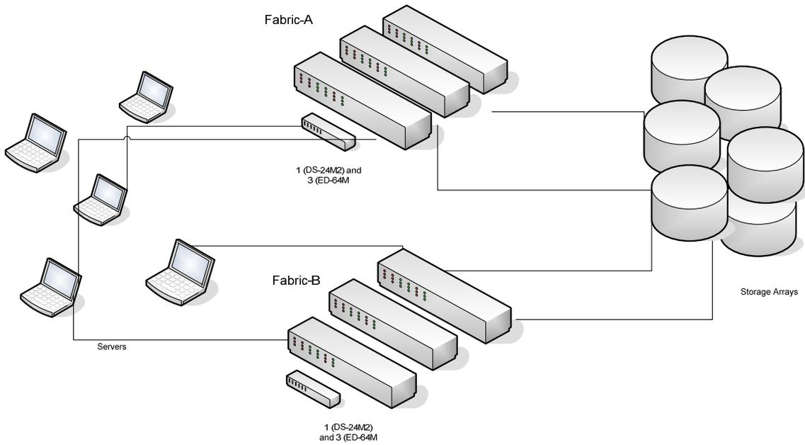
Backup the Zoning database of both SAN and print switch dumps of all switches. Have your Fiber cables run between two Islands but don't cable yet! Merge one fabric at a time.
